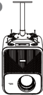
Adjust hanger angle to align with the hole and then tighten screws (4 pcs of UNC 1/4-20*3/8 )
